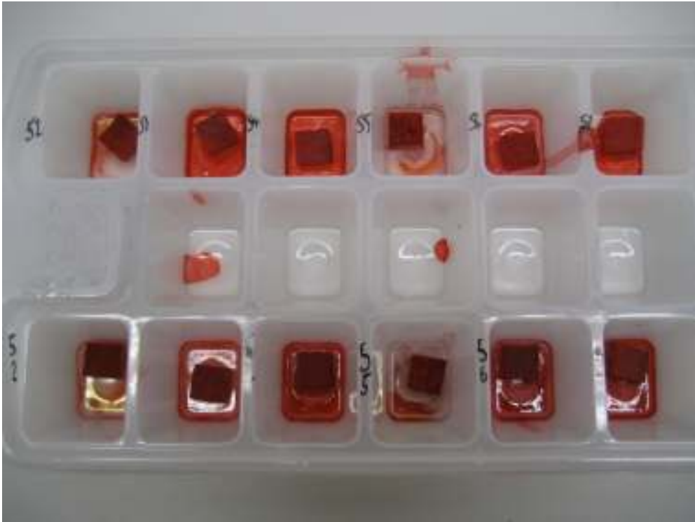
Image 3A-28; Control blocks – (0% cyclododecane + 0%, 5%, 10% consolidant)
