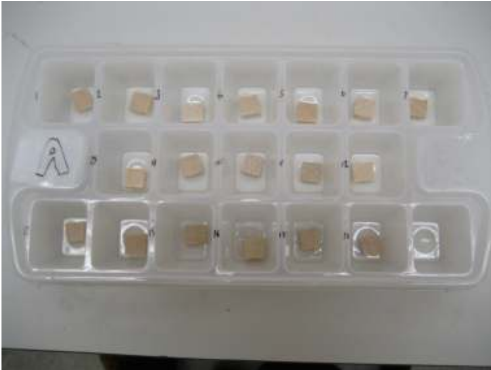
Image 3A-26; Control blocks – (0% cyclododecane + 0% consolidant)
