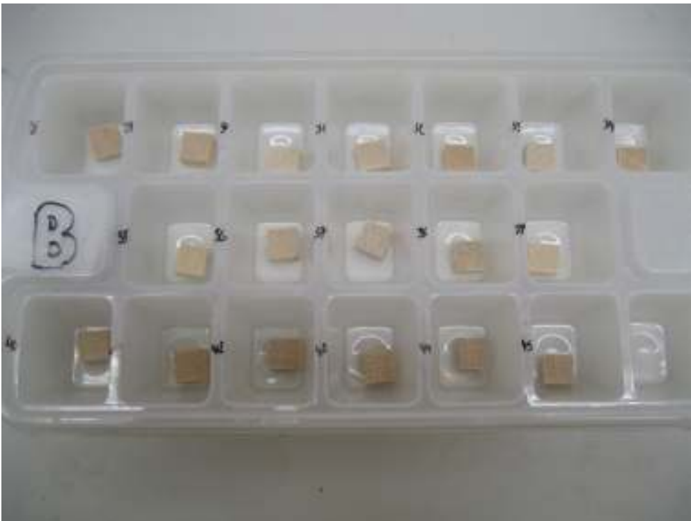
Image 3A-27; Control blocks – (0% cyclododecane + 0% consolidant)
